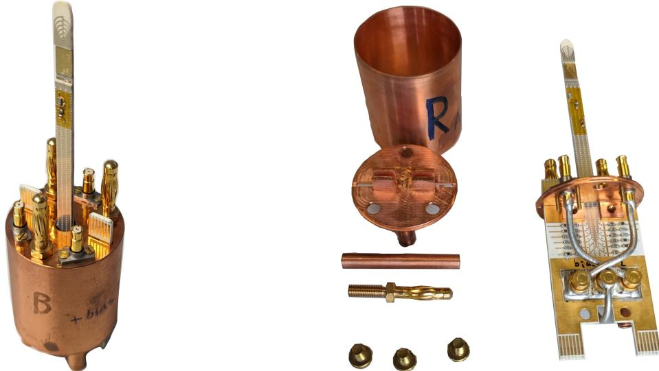
(a) The SMP-connectors lead to the rf-connectors on the sample PCB. The banana plugs are used for mechanical fixation, grounding and thermalisation. The visible PCI connectors are highlighted in **c**).
