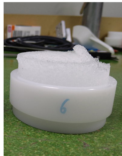
Figure 2.10: Left) Sketch of the laboratory setup for friction and compression tests. Right) A broken snow sample after a friction test.
