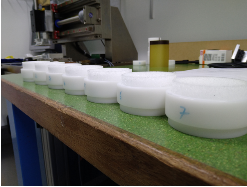
Figure 2.8: Fine-grained snow samples after a series of compression experiments.
