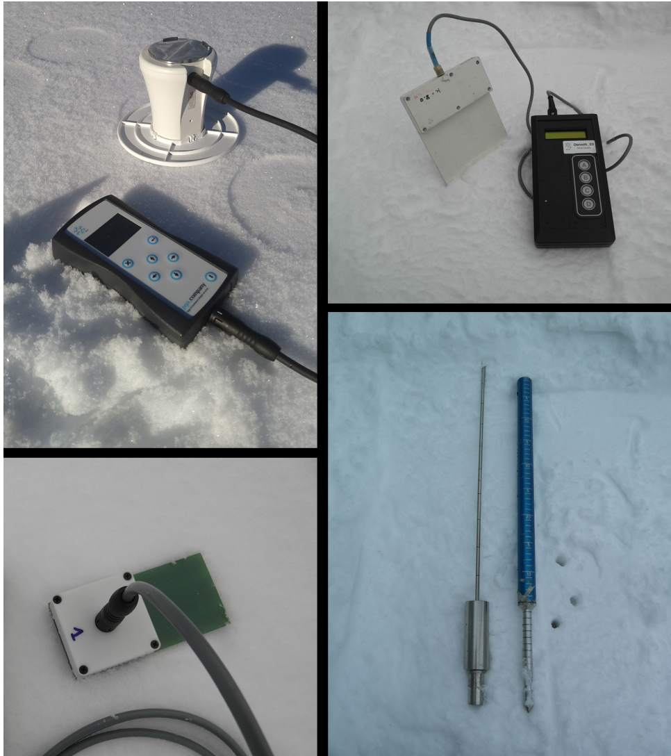
Figure 2.7: Instruments used to measure the snow properties: InfraSnow (top left), Dielectric sensors for LWC measurements (top right) and density (bottom left), and the adapted Swiss Rammsonde (bottom right).
