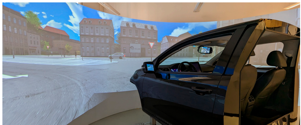
Figure 1. Driving simulator setup at the Institute of Human and Industrial Engineering (IFAB) at KIT.
