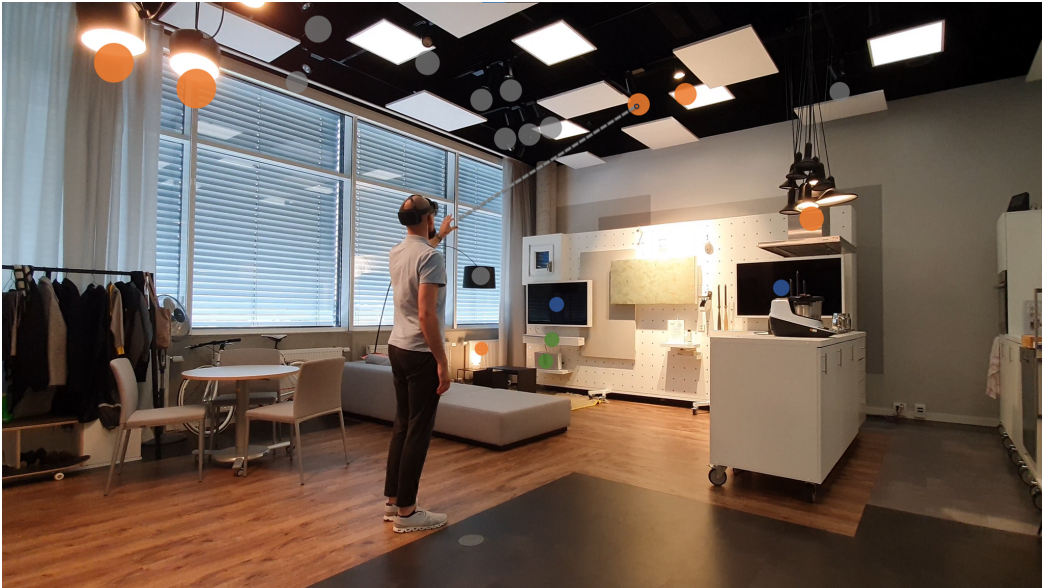
Figure 11.1.: Augmented Reality allows a direct interaction with Smart Home devices if their 3D position is known to the system. Our approach supports users with the spatial setup process of their Smart Home devices.
