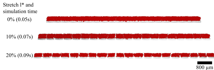
Figure 8. (Top): Loaded fiber consisting of fiber elements with 400 μm after completion of the loading phase with compact particle structure. (Bottom): Particle structure after 0.09 s and 0.07 s simulation time at a strain rate of 5/s. The asterisk represents the stretch percentage.
