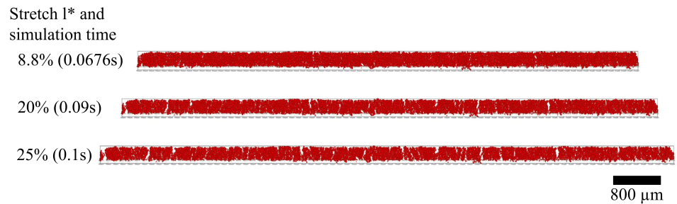
Figure 9. Loaded fiber consisting of fiber elements with 100 \mu\text{m} after completion of the loading phase with a compact particle structure. Snapshots of the particle structure after 0.0676 s, 0.09 s, and 0.1024 s stretching time with an elongation rate of 5/s. The asterisk represents the stretch percentage.
