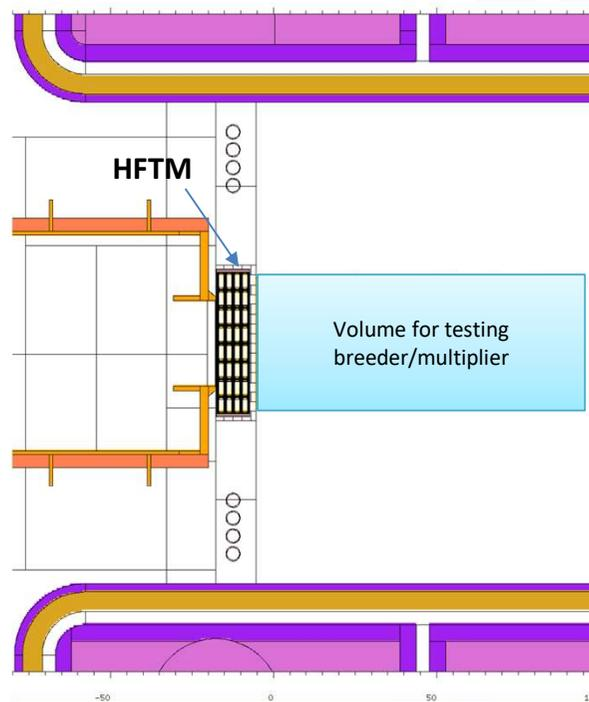
Volume for testing in Test Cell of IFMIF-DONES
