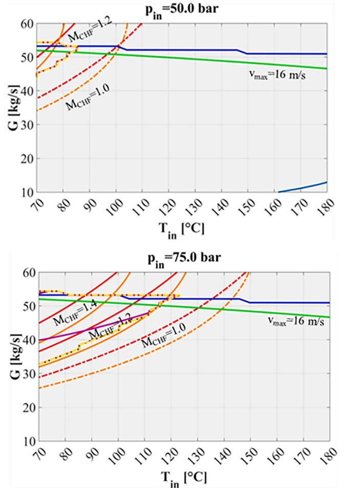
Fig. 9. Map of divertor (VTs in series) cooling circuit operating conditions for a maximum plasma heat flux of 30 MW/m<sup>2</sup>. Only the results at 16 m/s are reported.
