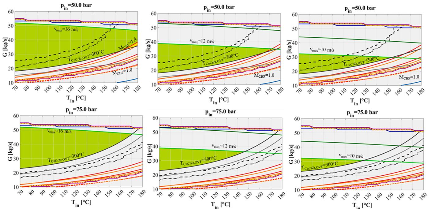
**Fig. 7.** Map of divertor (VTs in series) cooling circuit operating conditions for a maximum plasma heat flux of 10 MW/m<sup>2</sup>.
