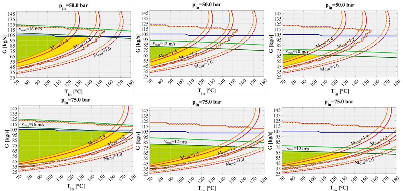
Fig. 10. Map of divertor (VTs in parallel) cooling circuit operating conditions for a maximum plasma heat flux of 20 MW/m<sup>2</sup>.
