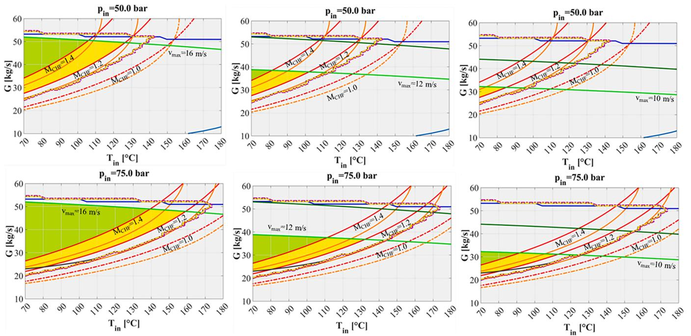
Fig. 8. Map of divertor (VTs in series) cooling circuit operating conditions for a maximum plasma heat flux of 20 MW/m<sup>2</sup>.
