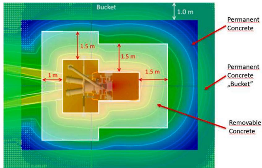
Fig. 4. Separation of biological shielding concrete.
