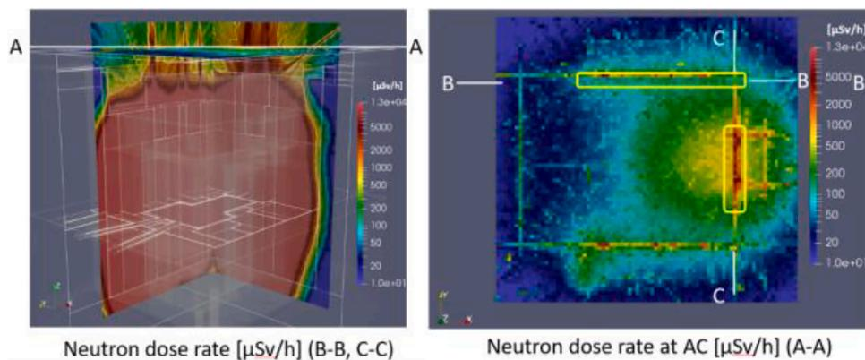
Fig. 6. Neutron dose rate [ $\mu\text{Sv/h}$ ] for the Case-1, plotted along the gaps B-B and C-C (left) and plotted in the AC at the upper surface of TCCP A-A (right). White contour line shows the value of 1000  $\mu\text{Sv/h}$ .
