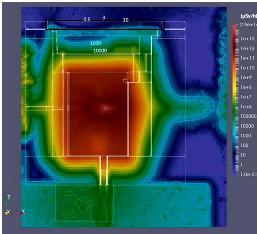
Fig. 7. Neutronics calculations using PE filling in the TCCP at the top of the TC.
