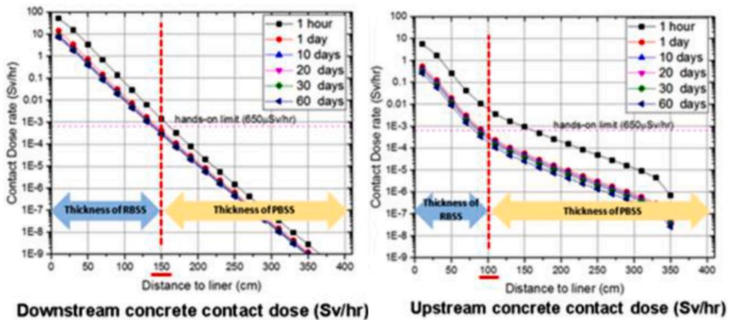
Activation of the concrete walls after 30 years of DONES operation (down- and upstream (+X and -X) directions)
