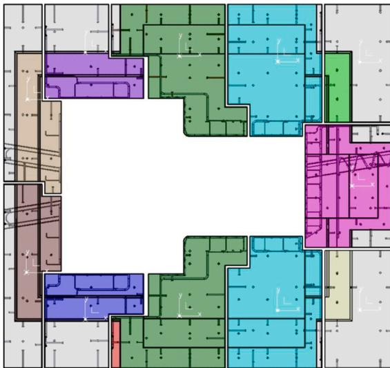
Fig. 11. RBSBs semitransparent top view with Center of Gravity (COG) points (white coordinate systems) of each block.
