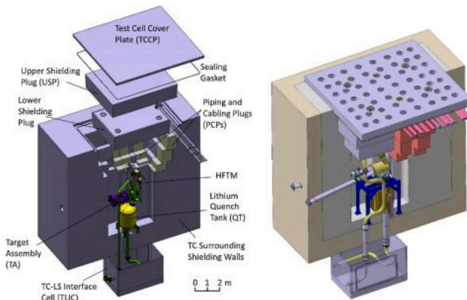
Fig. 1. Previous designs for the TC: IFMIF/EVEDA Coffin like setup (left); IFMIF-DONES monolithic concept (right).
