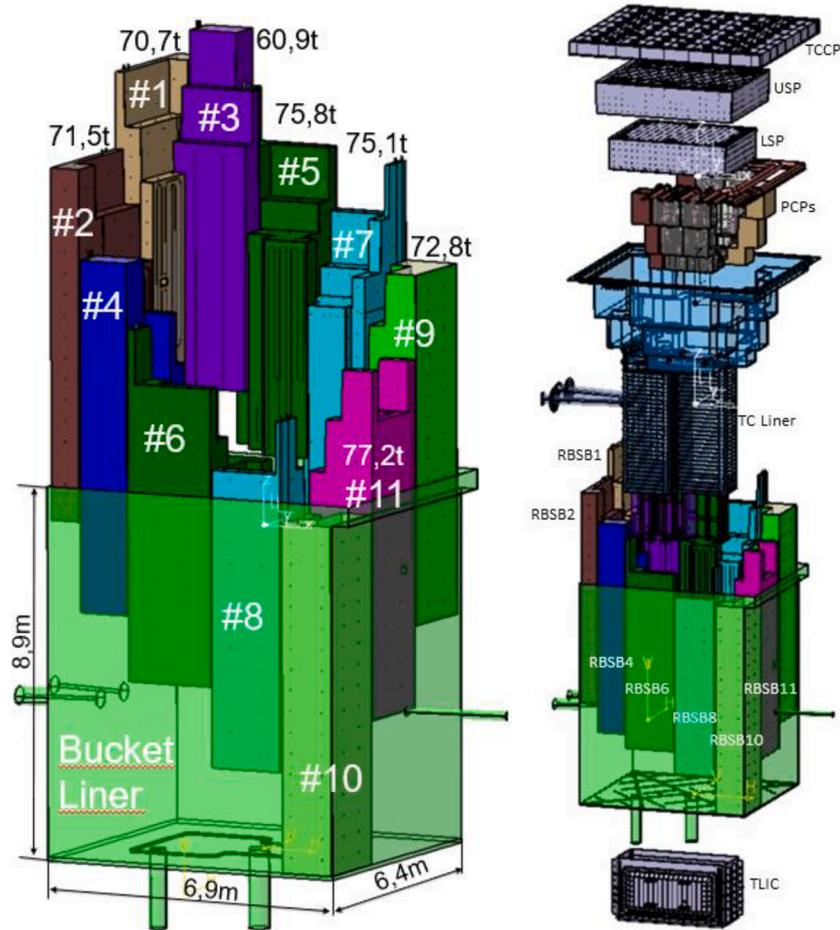
**Fig. 8.** Left side: RBSB #1 - #11 masses and dimensions (RBSBs are mirrored to the middle plane, so weights of RBSBs are identical as: #3=#4; #5=#6; #7=#8; #9=#10) Right side: whole TC 3D CAD model with all the components.
