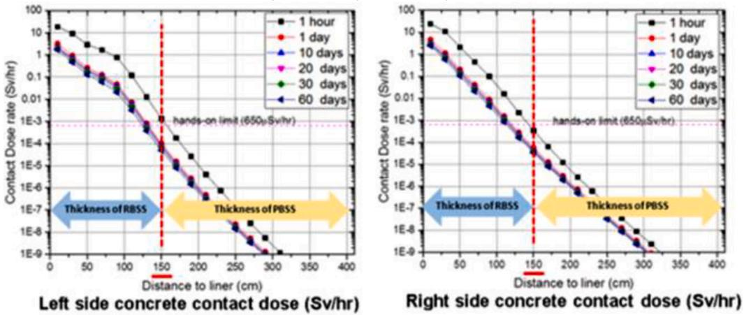
Activation of the concrete walls after 30 years of DONES operation (lateral side walls)
