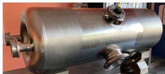
Figure 8: Picture of the naked high beta cavity before cryogenics tests.
