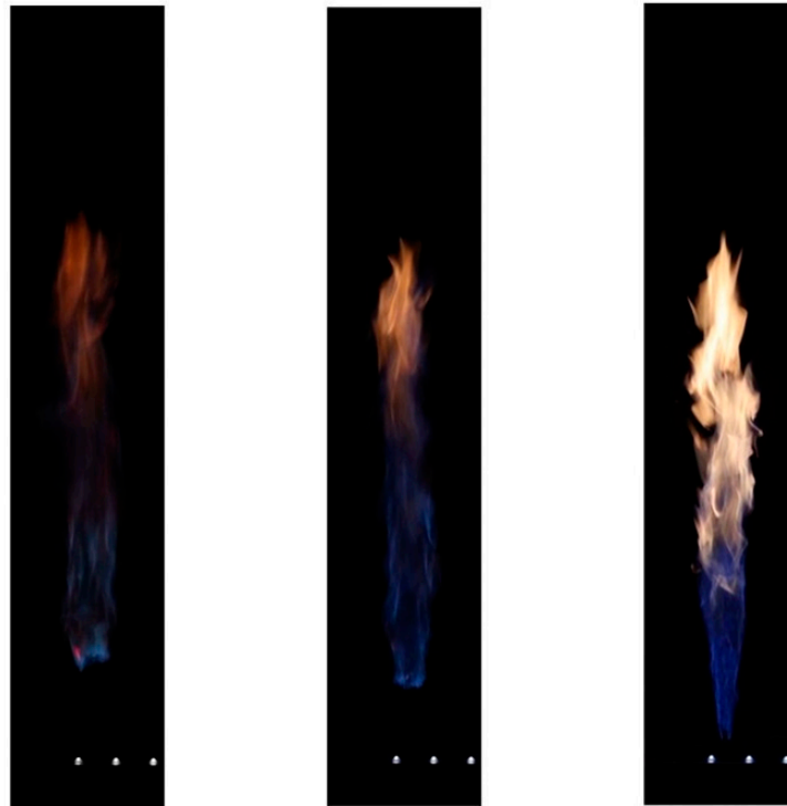
Figure 11. Flame images at a volume flow rate of 60 L/min. (a) 0 Vol.-% H 2 , (b) 20 Vol.-% H 2 , (c) 40 Vol.-% H 2 .
