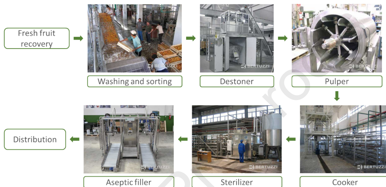
Figure 7 – Schematization of the process line to produce nectarines' puree
