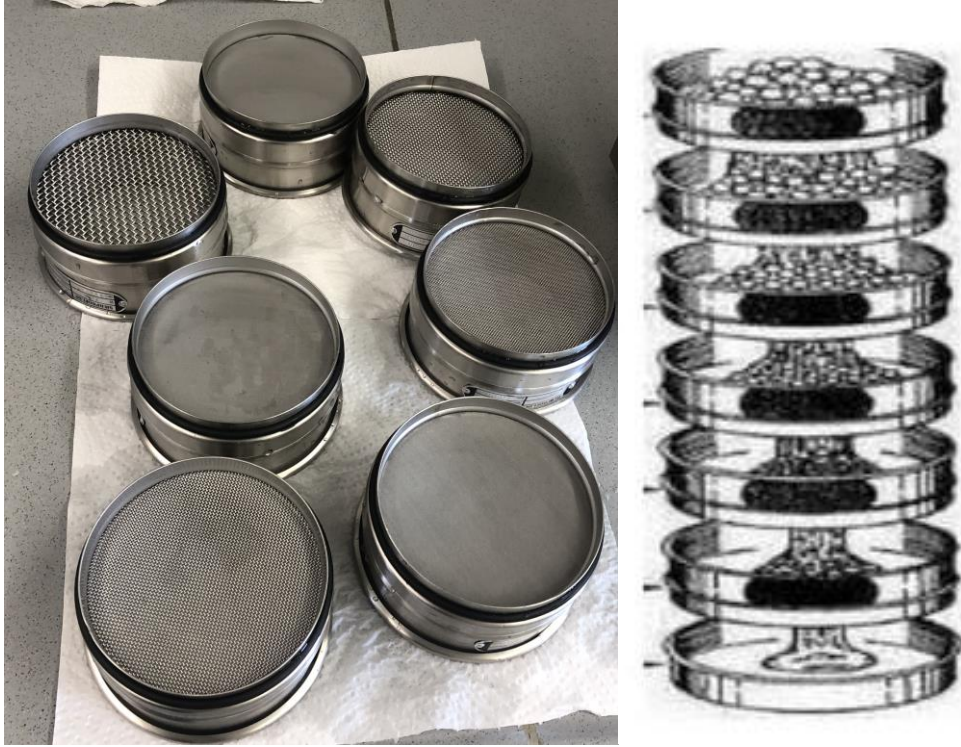
Figure 2.2 Sieves are used in the grain size measurement.
