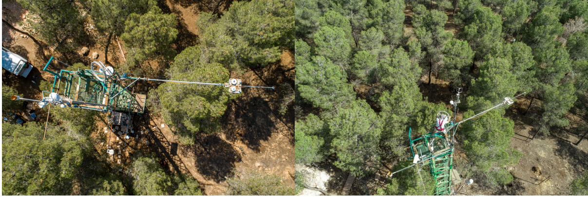
Figure 1.2: Flux tower instrumentation at Yatir Forest. The site consists of an eddy-covariance system (ECS), net radiometer, thermocouples, soil heat plate and rain gauge. ECS consist of a three dimensional sonic anemometer that measures wind speed and direction in three dimensions ( u , v , w ) and provides data on turbulence, and an infrared gas analyzer (IRGA) measures concentrations of CO_2 and H_2O vapor to calculate their fluxes. Net radiometer measures net radiation ( R_{net} ) as the difference between incoming and outgoing shortwave and longwave radiation. Thermocouples measure air and soil temperature. Soil heat flux plates measure ground heat flux ( G ), and rain gauges measure precipitation.
