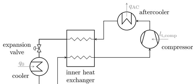
**Figure 1.** Single-stage cryogenic mixed-refrigerant cycle.
