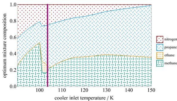
**Figure 3.** Change in optimum composition over different  $T_{cooler,in}$ .**Table 2.** Optimization parameters.
