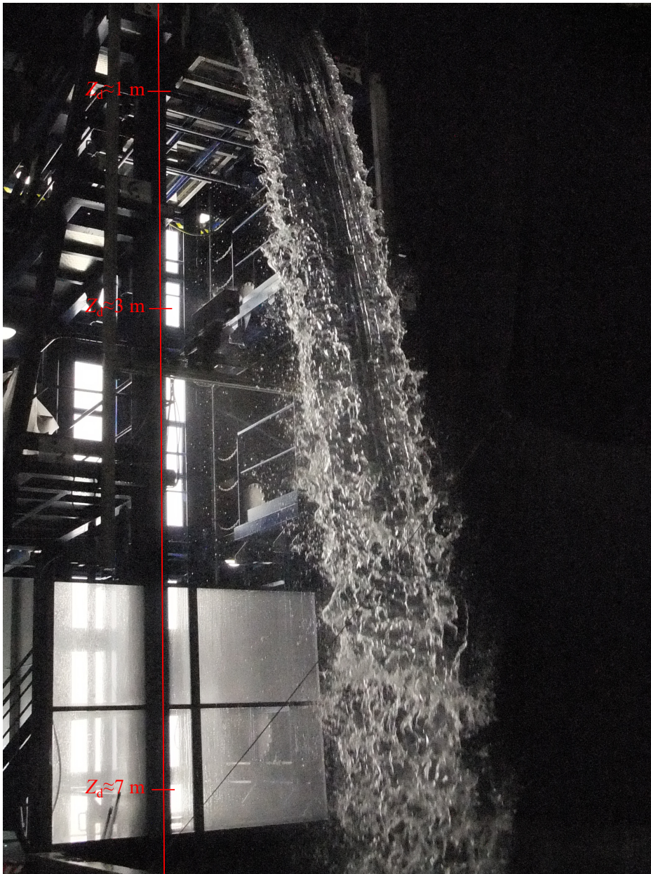
Fig. 1.2. Model setup of a sharp-crested weir at the laboratory of Électricité de France at Chatou. Specific folume flow rate \sim 0.2 \text{ m}^2/\text{s} . Threadlike deformations in the central area of the nappe surface can be observed. Image taken by Carsten Thorenz (2019) with an exposure time of 2 ms, showing about 7.5 m of the fall. More details on the setup in Bercovitz et al. (2018) .
