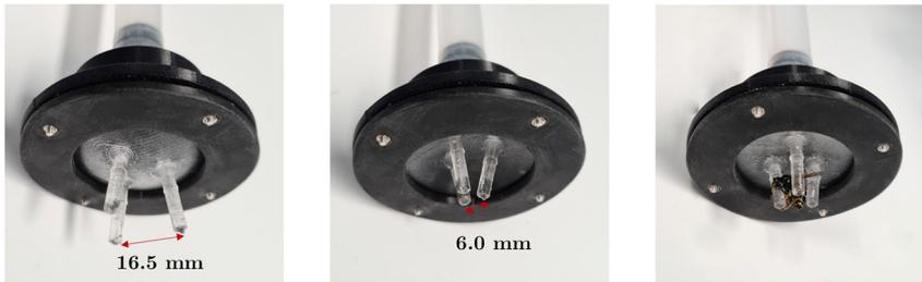
**Figure 3:** The mini-gripper with three fingers in its opened position (left), in its closed position (center), and while holding an insect (right).
