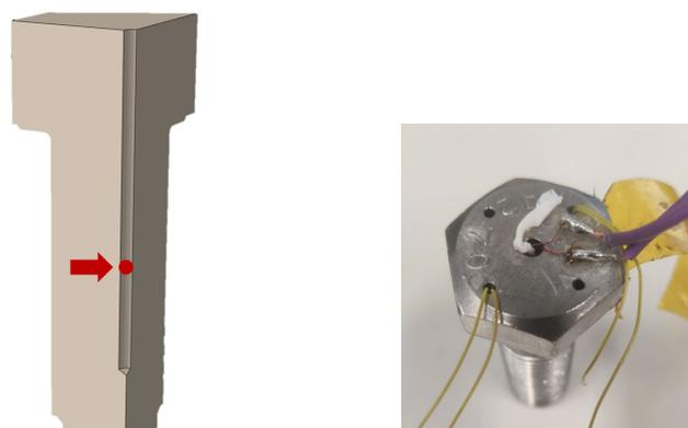
**FIGURE 9.** Node in the FE-model for strain evaluation (left) and cylindrical strain gauge applied in bolt with single cavity  $d_1 = d_2 = 2$  mm (right).
