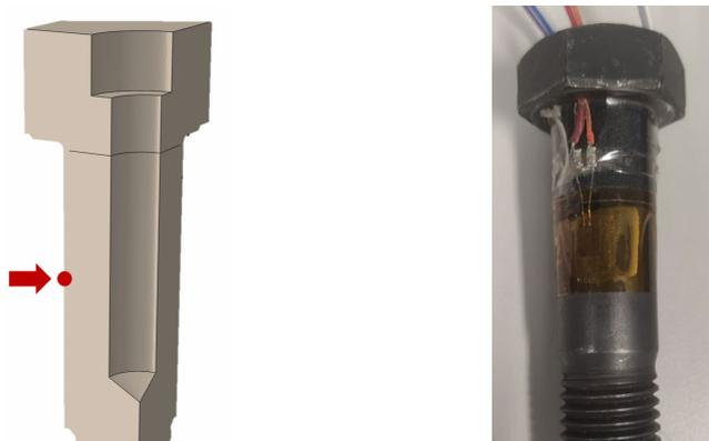
**FIGURE 8.** Node in the FE-model for strain evaluation (left) and applied strain gauges on the bolt with cavities  $d_1 = 10$  mm and  $d_2 = 13$  mm on the outside of the shaft, 3 strain gauges are spaced symmetrically in the cross-section (right).
