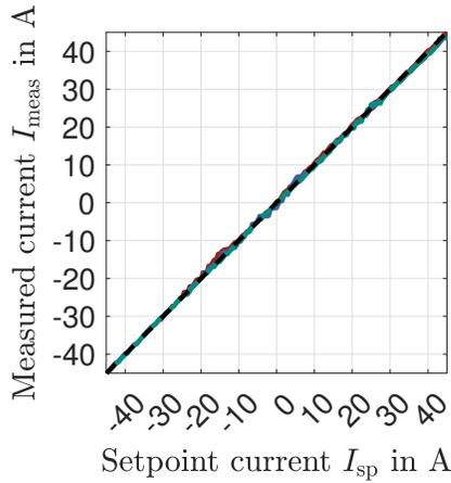
(c) Resulting open-loop transfer function with ESBOL.
