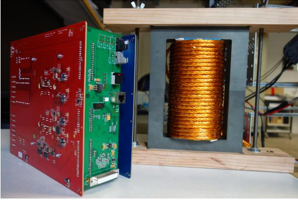
Fig. 5: Picture of one 40 kW DAB.
