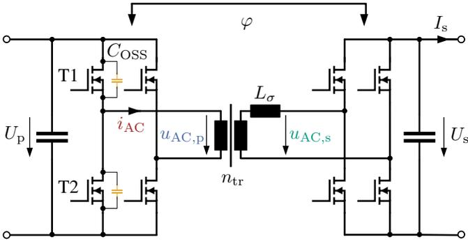
Fig. 1: Circuit diagram of a DAB with parasitic capacities  $C_{OSS}$  highlighted in orange across T1 and T2.
