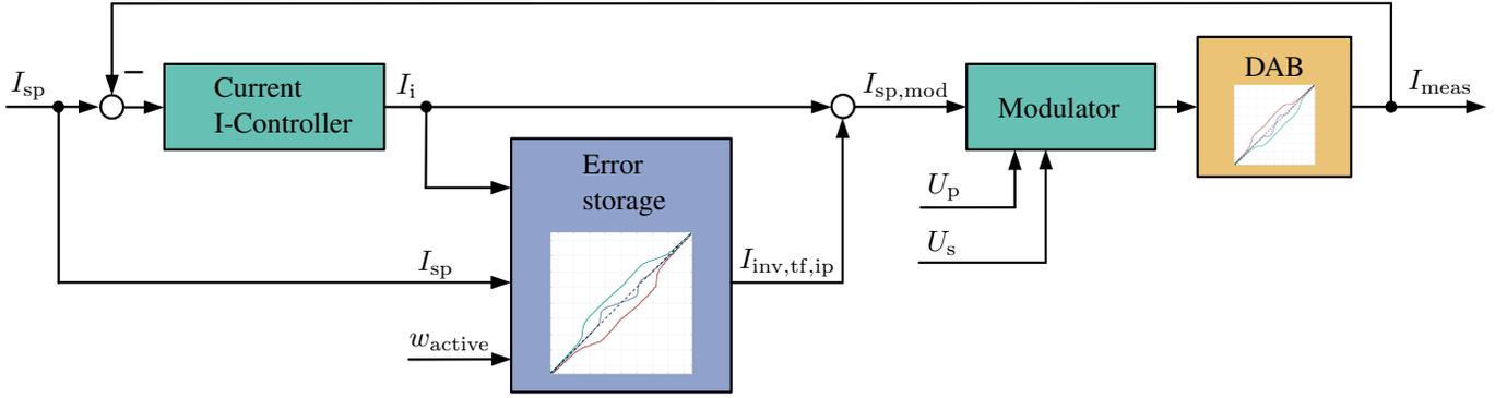
Fig. 3: Control structure of the current controller for the DAB. Without the Error storage system, a constant FF gain of 1 is implemented ( $I_{inv,tf,ip} = I_{sp}$ ).
