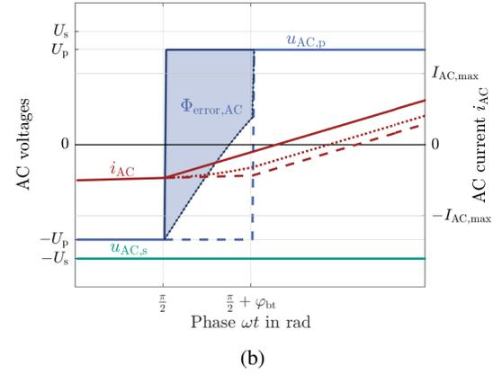
Fig. 2: Qualitative voltage and current waveforms of a DAB with SPS modulation. Here the DAB works in positive boost mode, i.e.  $I_s > 0$  A and  $U_s > U_p$ . In (a), the ideal waveforms are shown and in (b) a zoom of the non-ideal commutation process of the primary full bridge (dashed oval) is depicted. The blocking time  $T_{bt}$  can be represented as a blocking angle  $\varphi_{bt} = T_{bt} \cdot f_{sw} \cdot 2\pi$ .
