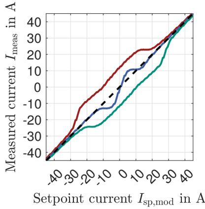
(a) Measured open-loop transfer function  $I_{\text{meas}} = G_{\text{DAB}}(I_{\text{sp}}) \cdot I_{\text{sp}}$ .
