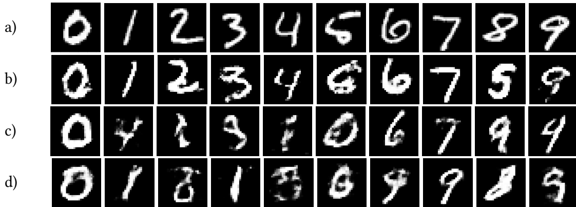
Figure 5.10.: Examples of (a) Original MNIST images, (b) recovered images in const memory mode (c) recovered images in decoupled memory mode, and (d) recovered images with the countermeasure applied.
