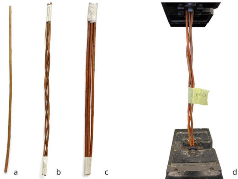
Fig. 15 Single willow stem (a), three willow stems braided (b), three parallel willow stems (c), braided willow in the testing machine (d)
