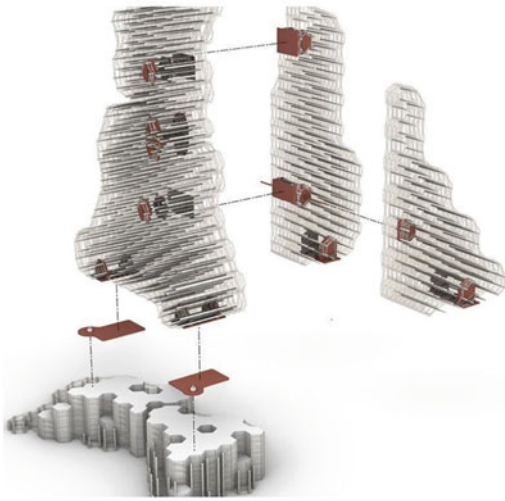
Fig. 23 Exploded view of a portion of InterTwig showing the joinery system
