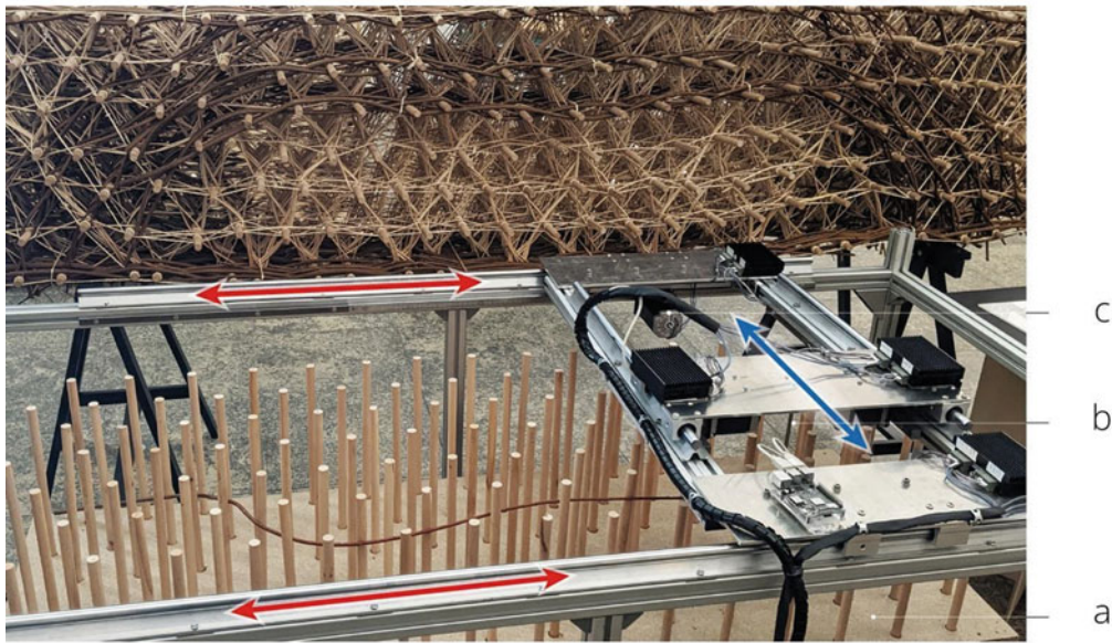
Fig. 12 View of the two-axis machine showing the bed of poles (a), the end effector (b) and the stepper motors (c)
