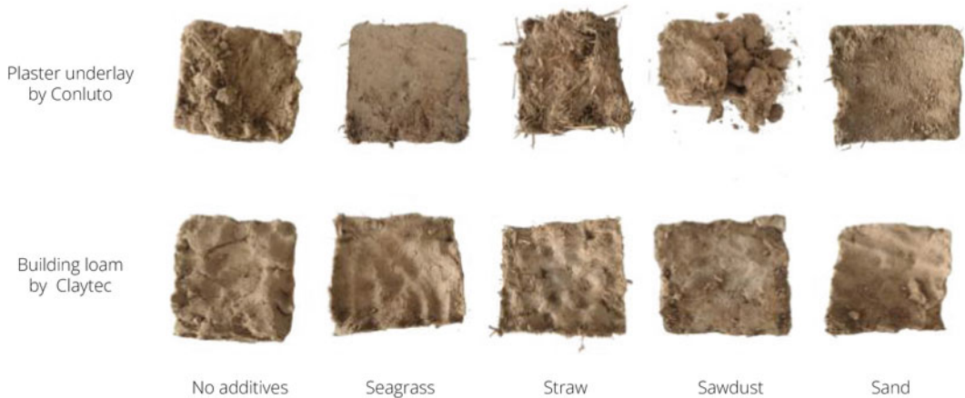
Fig. 5 Small prototypes combining commercially available earth products with different additives
