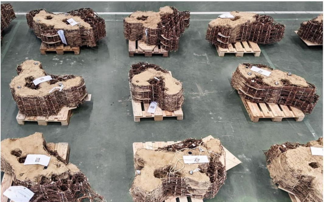
Fig. 22 Earth and willow components before assembly
