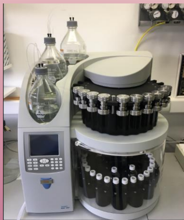
Accelerate solvent extractor (ASE) Cyclohexane: toluene 3:7
