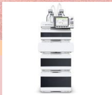
HPLC/FLD mobile phase acetonitrile : water 60:40
