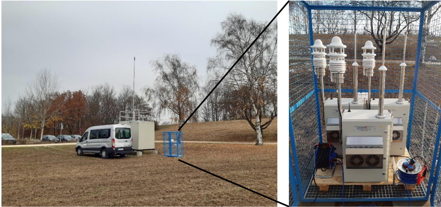
All three CPCs in the grid box next to the UFP measurement station of the Bavarian State Agency for Environment (University of Regensburg)
