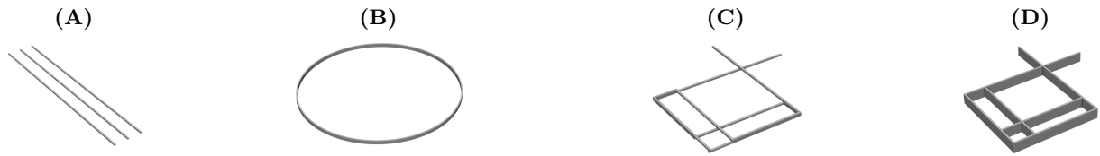
Figure A5.1 Designed models used during the Round robin - 3D printing test. (A) single layer line, (B) single layer circle, (C) two layer rectangle geometries, and (D) scaffold which equaled the rectangle geometry with several printed layers.
