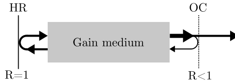
Figure 2.2: Schematic representation of a simple ideal laser resonator. The photons are amplified with each pass through the gain medium. The OC mirror is partially reflective which allows some of the photons to leave the resonator (adapted from [38]).
