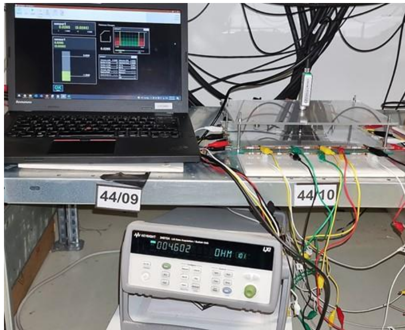
Figure 6.6. Photograph of the Li-ion battery thickness change monitoring setup. While the Li-ion cell is undergoing a charging and discharging cycle, a reference sensor, installed in the middle of the setup which is connected to a laptop (using the Keyence GT-Monitor 2 Test version software), is recording the displacement changes. Simultaneous to reference data and Li-ion battery cycling, the real-time
