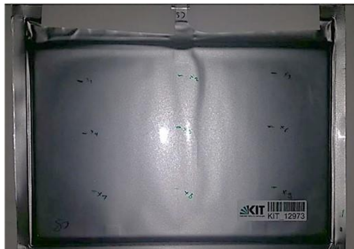
Figure 6.12. Photograph of the Li-ion battery pouch cell used in this work. Spots used for static thickness measurements are marked with x from top left x1 to bottom right x9. The thickness of the cell in the static mode is measured once in a 0% state of charge and once in 100% (not during cycling, but in a fixed state of charge).
