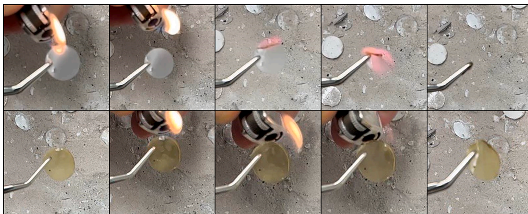
Fig. 6. Results of flame tests of PEO with 20:1 EO/Li ratio of LiTFSI (top) and PI 85 -PEO 15 with 70 wt% LiTFSI (bottom).
