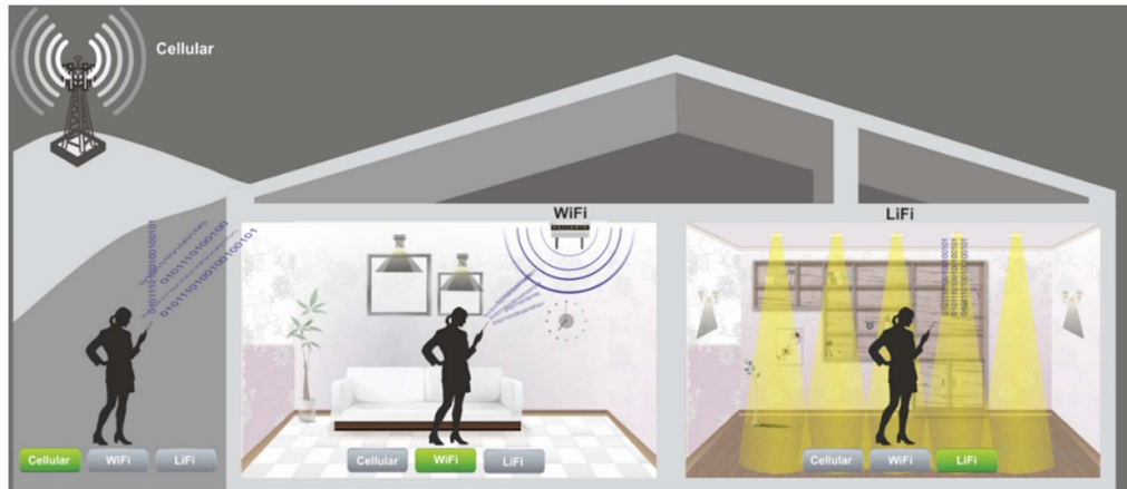
Figure 35. VLC is positioned as a complementary wireless access solution to radio-based cellular and WiFi systems, releasing the pressure on highly congested RF spectrum.
