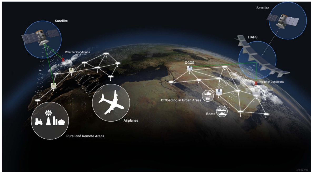
Figure 33. Hybrid very high throughput satellite networks with site diversity and HAPS relaying.
