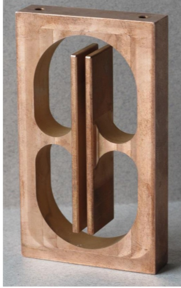
Figure 3.5: Ring loop resonator design developed by [54], where the function of the resonator was to maintain a high magnitude E_2 while reducing the stray magnetic fields produced. The dimension of the resonator in length and width was 70 mm by 40 mm respectively. (Reprinted from [54] fig. 5(A), with the permission of AIP Publishing).
