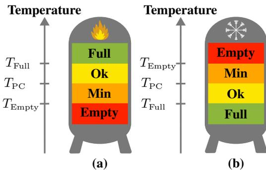
Fig. 3 Integration of TES into EMS, the four zones for (a) heating TES and (b) cooling TES based on full, empty, and phase change temperatures.
