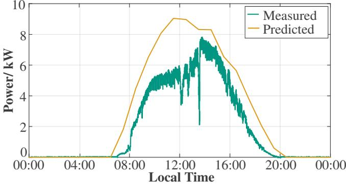
Fig. 4 PV power prediction for a sunny day compared to the measured values.
