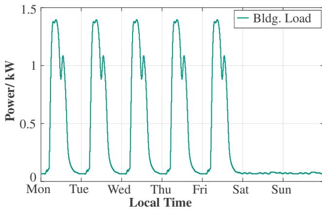
Fig. 2 One week electrical power consumption by the building, generated based on the standard load profile from BDEW [15]
