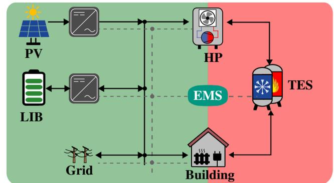
Fig. 1 System layout with solid connection lines depicting the physical connection and dotted lines depicting the communication between the components
