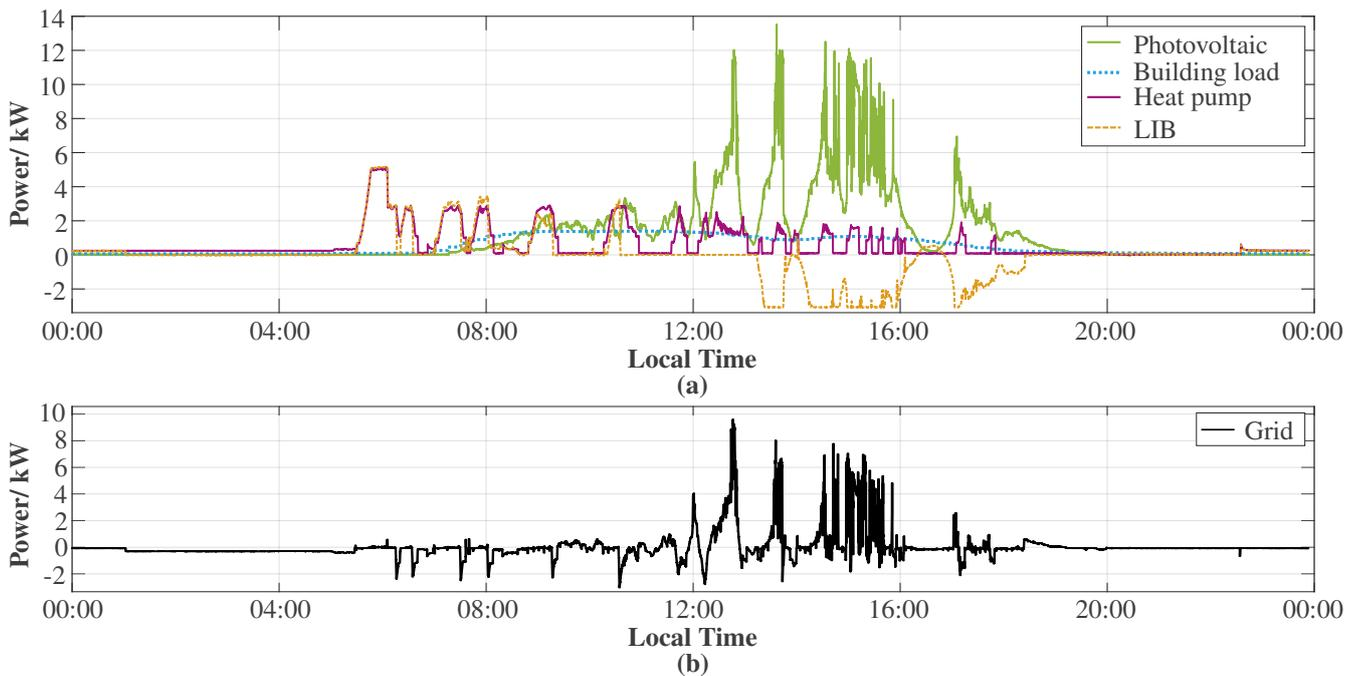
Fig. 6 Operation of the PV-HP System with EMS on a normal day with moving clouds - April 25, 2024. (a) power curve of system components; (b) power curve of the grid
