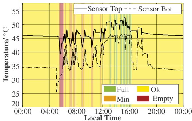
Fig. 8 Temperature curve in the upper and lower area of the heating TES with visualisation of the TES states from an EMS perspective.
