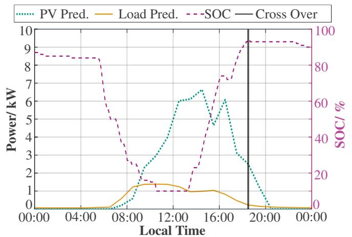
Fig. 7 SOC curve of the LIB with optimised charge management based on the intersection of load and PV forecast.
