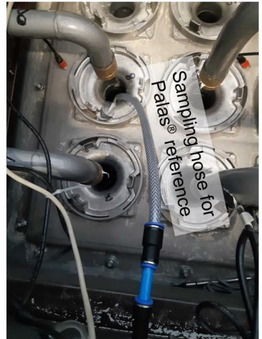
Appendix 1 – Setup of reference measurement employing the Palas® system at individual filter bags on the clean gas side of the filter
