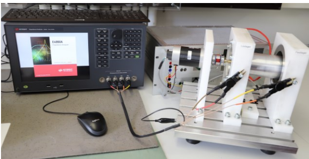
Figure 4: Measurement setup to determine the bearings impedance
