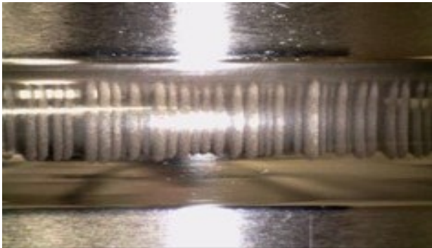
Figure 2: Corrugated patterns at the outer raceway
