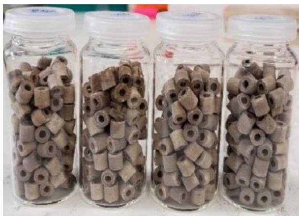
Figure 5: Photograph of four batches of synthesized Pt/Al 2 O 3 with optimized immobilization onto hollow cylinders. Synthesis conditions: Batch procedure, PVP:Pt ratio = 5 g PVP g Pt -1 and NaBH 4 :Pt ratio = 0.31 mol NaBH 4 mol Pt -1 .
