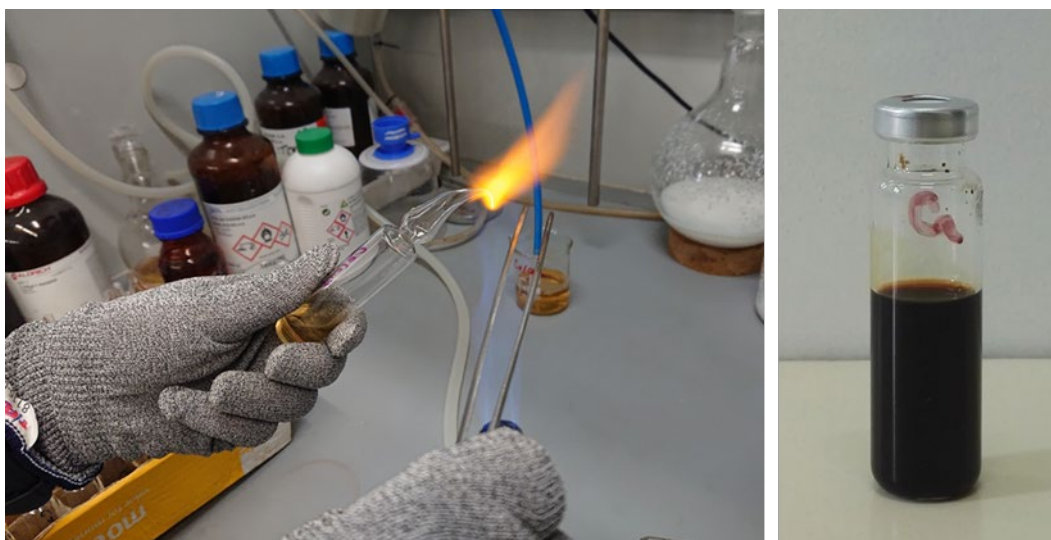
Figure 3 : Sealing of glass ampoules (left) and a crimp vial (right) with samples for radiolysis and hydrolysis
