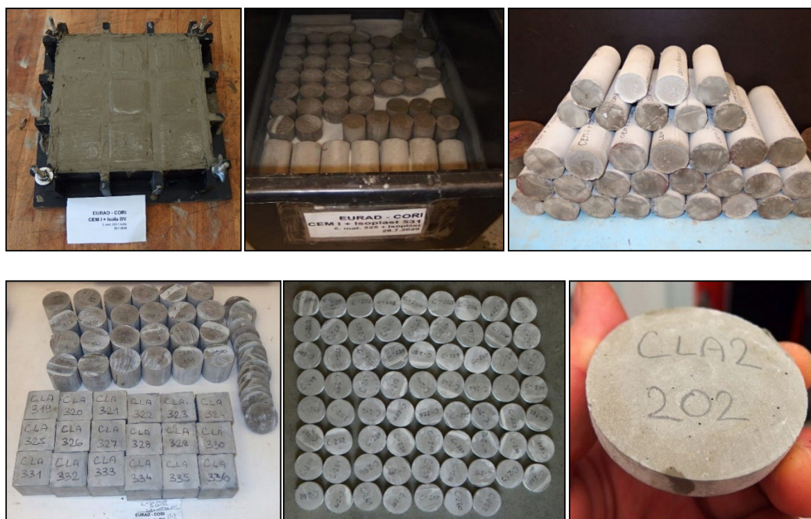
Figure 3: Preparation of CEM I paste samples.
