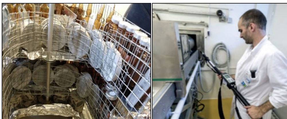
Figure 4: HCP and Richard concrete samples in front of the irradiator (left) and dosimetry measurement in the radiation chamber during door closing (right).
