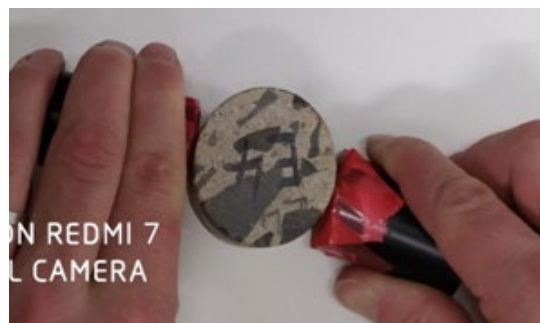
Figure 11: Measurement of the Richard concrete sample using the ultrasonic pulse method (by Pundit PL200).
