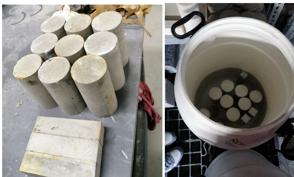
Figure 1: Batch 1. Aspect of the specimens and curing procedure
