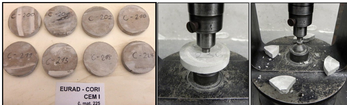
Figure 5: A punch test on CEM I HCP discs
