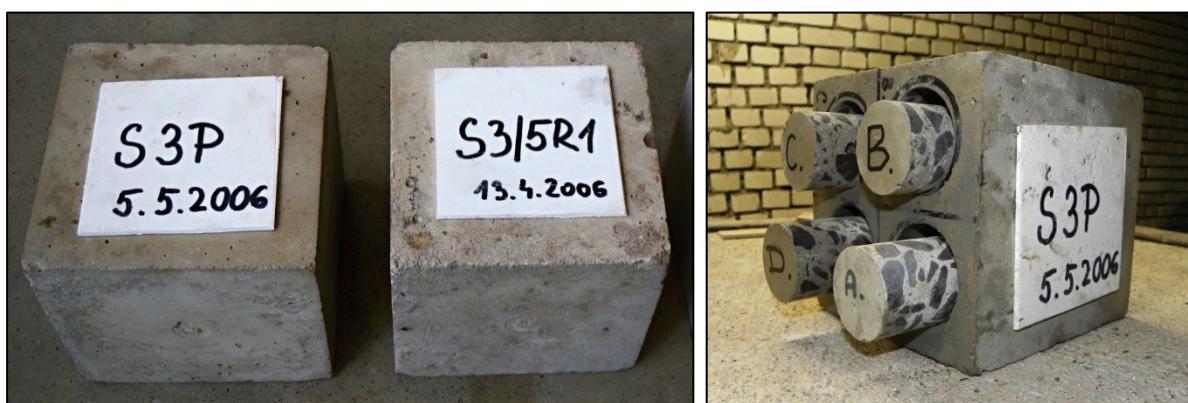
Figure 1: Two cubes of structural concrete from the Richard LLW/ILW repository (left) and cores drilled from S3P (right).
