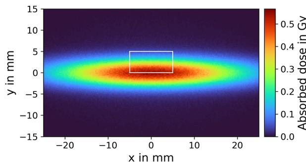
Figure 7: Simulated 2D absorbed dose profile for an exposure time of  $t = 11 \text{ s}$  and a photon beam with Gaussian shape and an energy of 16 keV.
