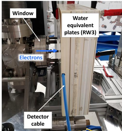
Figure 2: Depth dose curve measurement setup at FLUTE. The electrons pass through a 150  $\mu\text{m}$  stainless steel window into air, where they then traverse a water phantom with the embedded detector.
