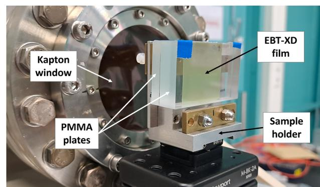
Figure 4: EBT-XD irradiation setup at the IMAGE X-ray beamline at the synchrotron KARA. Films placed between PMMA plates serve as a water phantom substitute.
