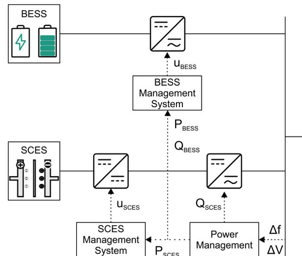
Fig. 8. Example of HESS management system architecture.
