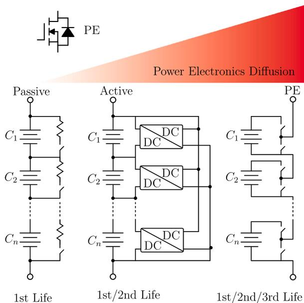
Fig. 2. Evolution of BMS towards fully PE-based technology.
