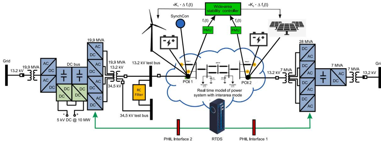
Fig. 15. Conceptual diagram of two-area PHIL experiment.
