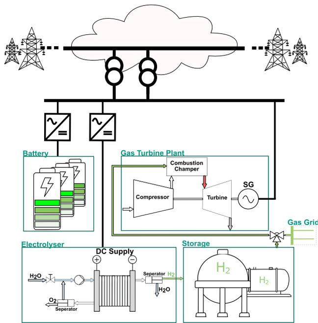
Fig. 11. The main elements of H2REB project.
