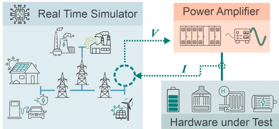
Fig. 12. Power hardware in the loop concept.
