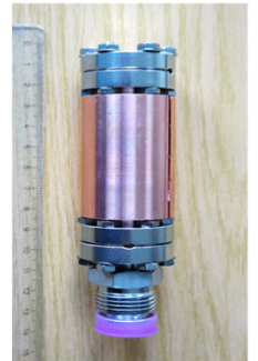
Vacuum fired specimen container 13 cm3
