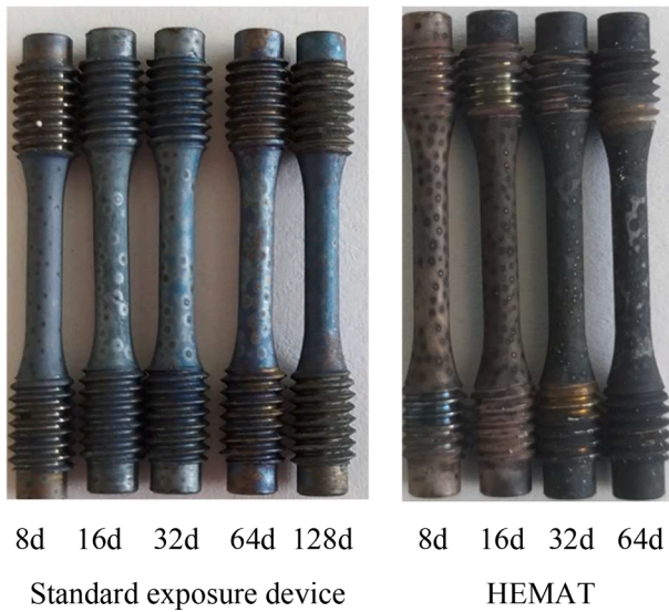
Fig. 8. Comparison of sub-sized LCF samples subjected to a ceramic breeder environment for different durations. Left: samples aged in a standard exposure device, right: samples aged in HELOKA HEMAT.
