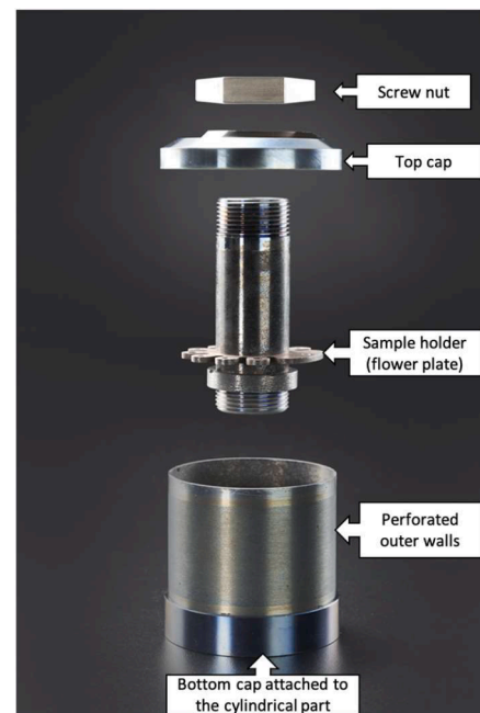
Fig. 1. Constituent parts of a canister (without samples).
