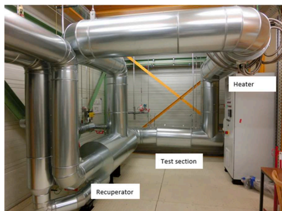
Fig. 3. High temperature part of HEMAT loop.
