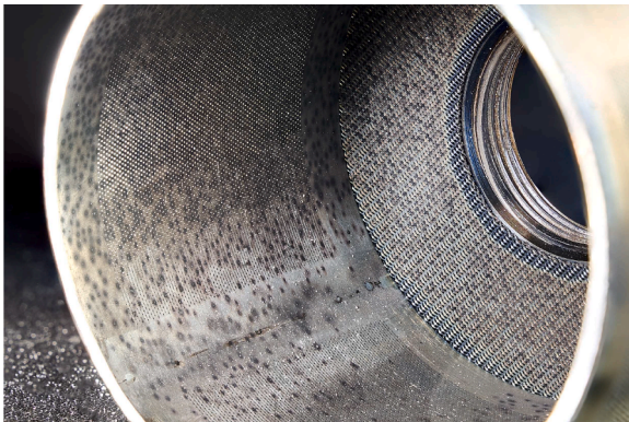
Fig. 5. Contact points of the pebbles with the canister side wall made from EUROFER, after 8 days exposure time.
