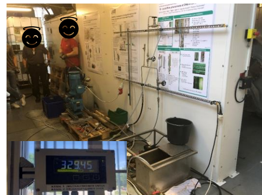
Figure 1: Preparation of the system for the pressure test. Right: High-pressure pump and pressure measurement technology for the application of the test pressure, left: Snapshot of the leak at the lower test section flange at approx. 250 bar
