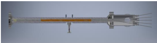
Figure 2: Longitudinal cut through the planned rod bundle deformation test section in EU-Project PATRICIA with the deformation piston in the center.
