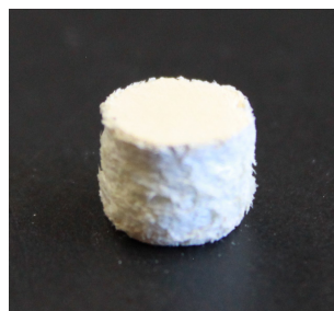
Figure 4: Foam sample filled at the top and bottom surface with fine filler for better load distribution and introduction into the closed-cell inner section of the foam.
