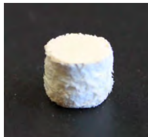
Figure 4: Foam sample filled at the top and bottom surface with fine filler for better load distribution and introduction into the closed-cell inner section of the foam.
