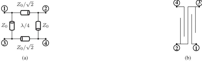
Figure 4.2: Corresponding ports,  $P_2$ : in,  $P_1$ : out1,  $P_3$ : out2,  $P_4$ : iso for (a) Branch-line coupler. (b) Lange coupler. [2] © IEEE
