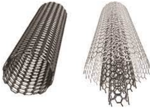
Fig. 3. On the left you can see a SWCNT and on the right a MWCNT .
