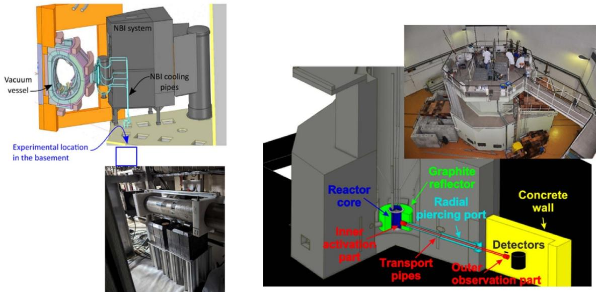
**Figure 18.** (left) JET water activation experiment: NBI duct scraper cooling loop equipped with shielded gamma ray detectors located in the basement under Octant 4; (right) KATANA, the new closed-water activation loop at JSI TRIGA Mark II research reactor. Adapted from [108], Copyright 2021, with permission from Elsevier. Adapted from [109], Copyright 2023, with permission from Elsevier.
