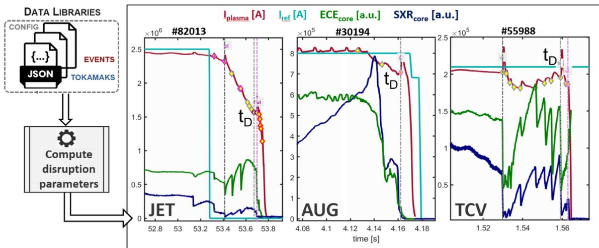
**Figure 9.** Automatic calculation of disruption characteristic times for JET, ASDEX-Upgrade (AUG) and TCV experiments based on the correlation of various quantities, where  $I_{\text{plasma}}$  is the plasma current,  $I_{\text{ref}}$  is the reference plasma current,  $ECE_{\text{core}}$  and  $SXR_{\text{core}}$  are proxies for the core temperature based respectively on electron cyclotron emission and on soft x-rays. Reproduced from [12]. The Author(s). CC BY 4.0.
