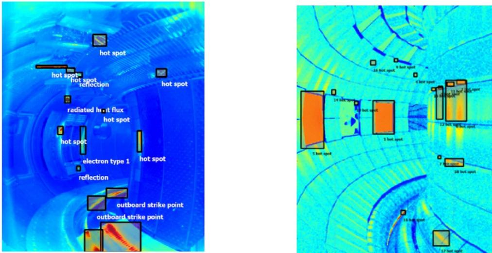
**Figure 5.** (left) WEST wide-angle IR images and automatic thermal events detection [Reprinted from [38], Copyright 2023, with permission from Elsevier]. (right) ITER simulated IR image where thermal events are automatically detected using algorithm trained on WEST data.
