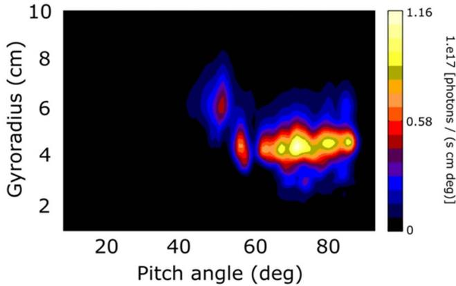
**Figure 7.** Simulated FILD measurements of the velocity-space distribution (as a function of gyroradius and pitch angle) of the escaping ions for ITER baseline scenario obtained with the synthetic diagnostic FILDSIM combined with an ASCOT simulation for calculating the fast ion losses at the diagnostic location.
