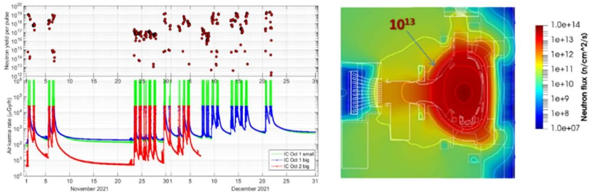
**Figure 14.** (left) measured neutron yield for each plasma shot (upper plot) and air kerma rate (in micro-gray per hour) versus calendar date during the last two months of DTE2; (right) neutron flux map in octant 1 for the JET D–T pulse 99 971 calculated by MCNP radiation transport code; contour line at  $10^{13} \text{ n cm}^{-2} \text{ s}^{-1}$  has been highlighted.
