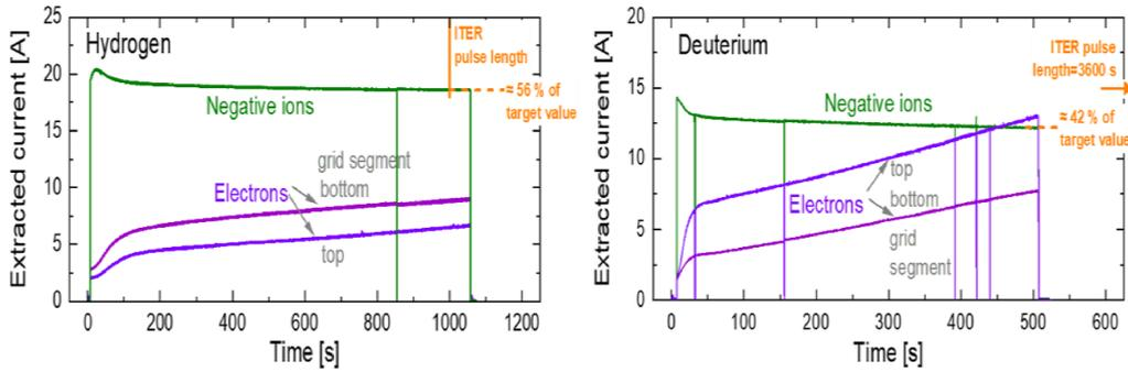
**Figure 11.** ELISE time traces of the extracted negative ion current and co-extracted electron current measured separately for the top and bottom segment of the extraction system during long pulses with the new CW high-voltage power supply in hydrogen (left) and deuterium (right). Reproduced from [13]. The Author(s). CC BY 4.0.
