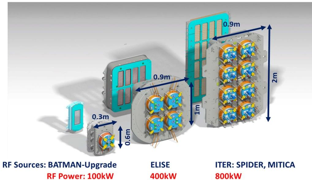
**Figure 10.** The RF sources development in a step-ladder approach towards ITER with the support of the EUROfusion facilities BATMAN Upgrade and ELISE. Adapted from [67], with permission from Springer Nature.
