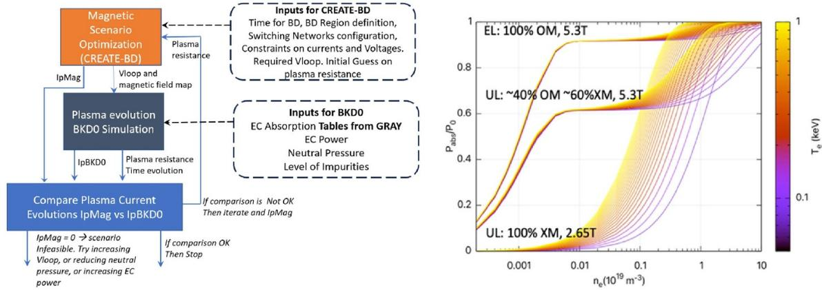
**Figure 2.** (left) General layout of the CREATE-BD/BKDD/GRAY coupling scheme for breakdown simulations; (right) ITER simulation: EC absorption for O-mode (OM) injection from EL and UL at 5.3 T and X-mode (XM) injection from UL at 2.65 T. Reproduced from [7]. The Author(s). [CC BY 4.0](#).
