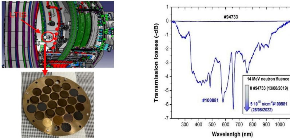
**Figure 15.** (Left) CAD drawing of the JET vessel section with the LTIS; picture of the LTIS sample holder taken after DTE2 with the irradiated ITER sample materials and dosimetry foils. (right) Transmission losses of silica optical fibers optics versus wavelength (nm) after neutron exposition during JET D–D, D–T and T–T experimental campaigns. The losses are normalized to the initial value before D–T neutron pulses (pulse #94733).
