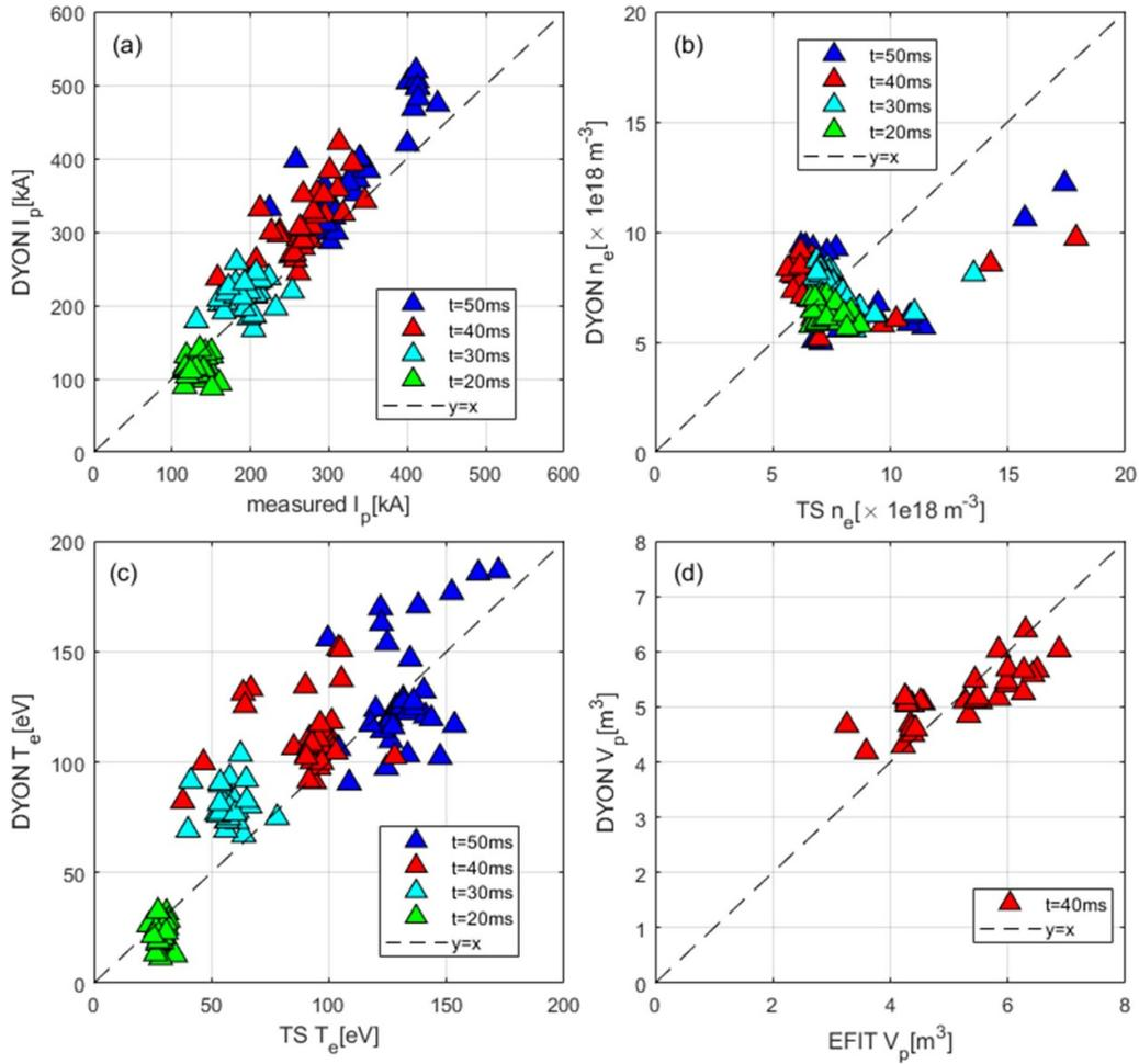
**Figure 1.** Statistical comparison between DYON plasma burn-through modeling calculation and MAST measurements: (a) plasma current, (b) electron density, (c) electron temperature and (d) plasma volume. Reproduced from [22]. The Author(s). [CC BY 4.0](https://creativecommons.org/licenses/by/4.0/).
