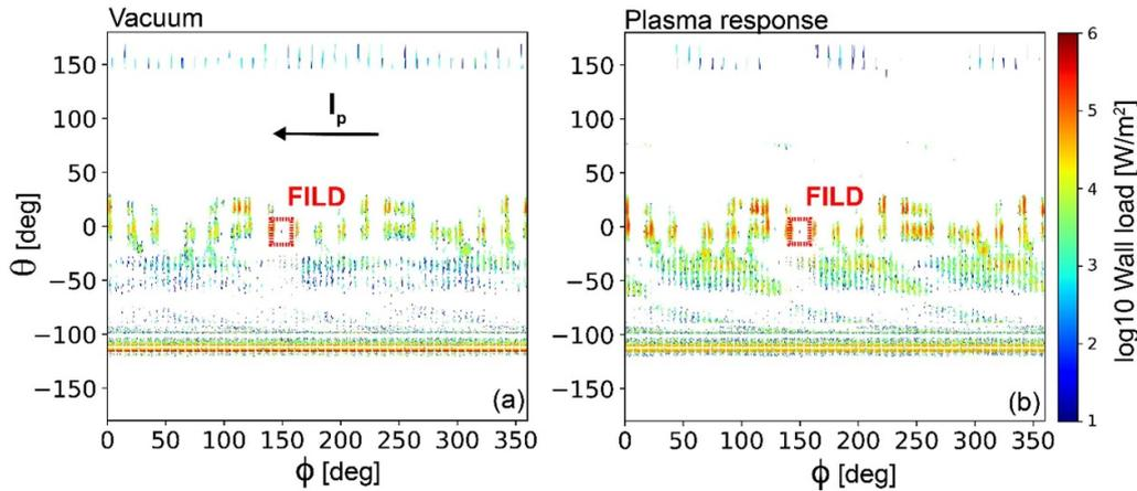
**Figure 6.** Simulated alpha-particle heat loads on the ITER first wall versus toroidal angle  $\phi$  and poloidal angle  $\theta$  in the presence of  $n = 3$  magnetic perturbations for the baseline 15 MA scenario with two different assumptions: (a) the vacuum and (b) including the plasma response to the applied perturbation on the fast ion losses. The location of the FILD head is indicated with a brown box.
