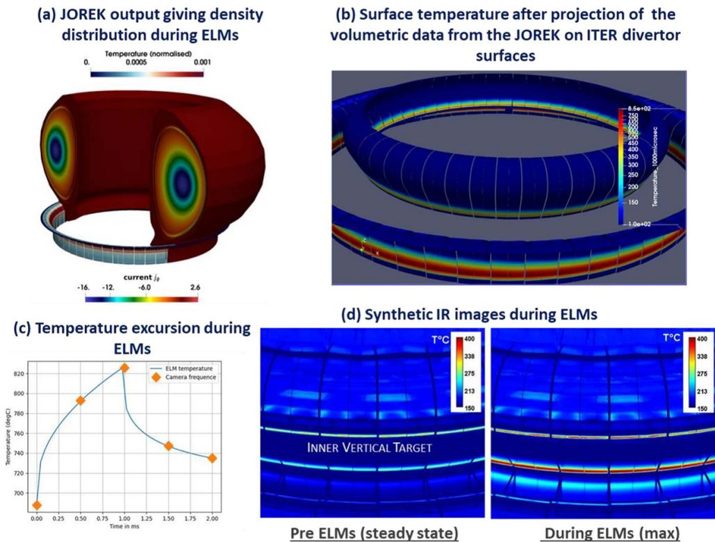
Figure 4. ITER simulation of transient ELMs in the IR synthetic diagnostic: (a) density distribution computed from JOREK, (b) volumetric data from the JOREK projected onto first-wall divertor surfaces, (c) temperature evolution, (d) synthetic images during ITER ELMs [10].
