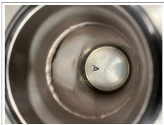
Figure 3. Picture of evaporated sodium in the condenser after an experiment.
