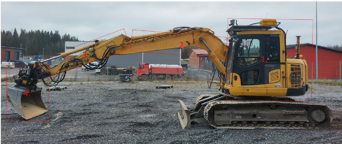
**Fig. 3** Excavator used in data collection. In the picture, cabin (1), boom (2), arm (3), and bucket (4) are highlighted with red boxes (Molaei et al. 2022)
