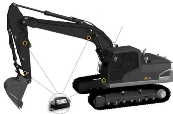
Fig. 5 The configuration of IMUs on the excavator
