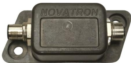
Fig. 4 The IMU used in the data collection phase
