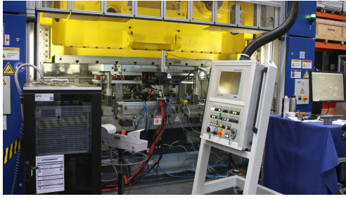
(a) Servo-hydraulic press with a mounted progressive die and the PLC.
