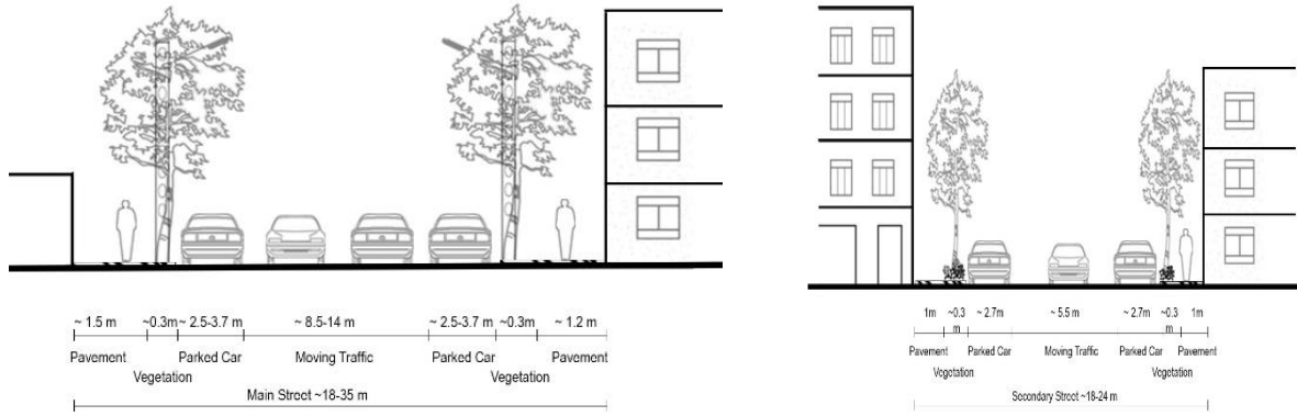
Figure 4.37. Street section 1-1 (left) and section 2-2 (right) from main and secondary streets in the Darrous Neighborhood
