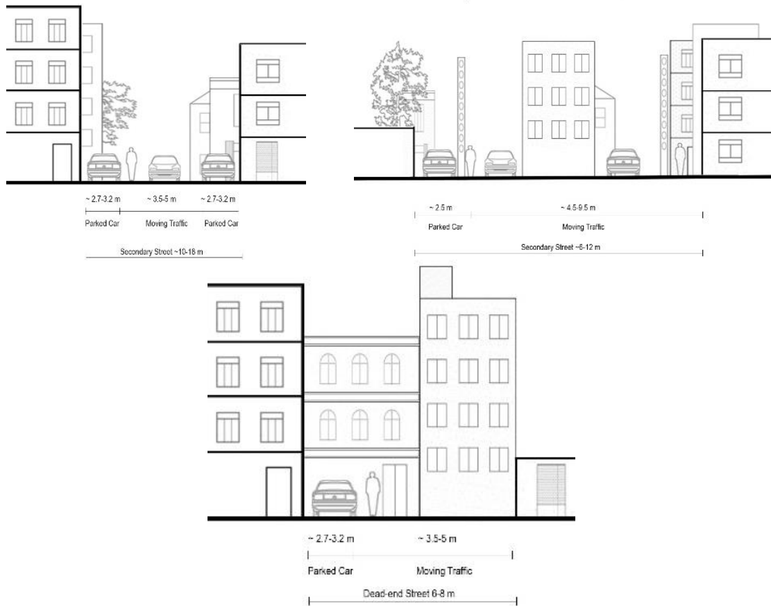
Figure 4.29. Street sections 3-3 (above left), 4-4 (above right), and 5-5 (below) from secondary and dead-end streets in the Dr. Hooshyar Neighborhood
