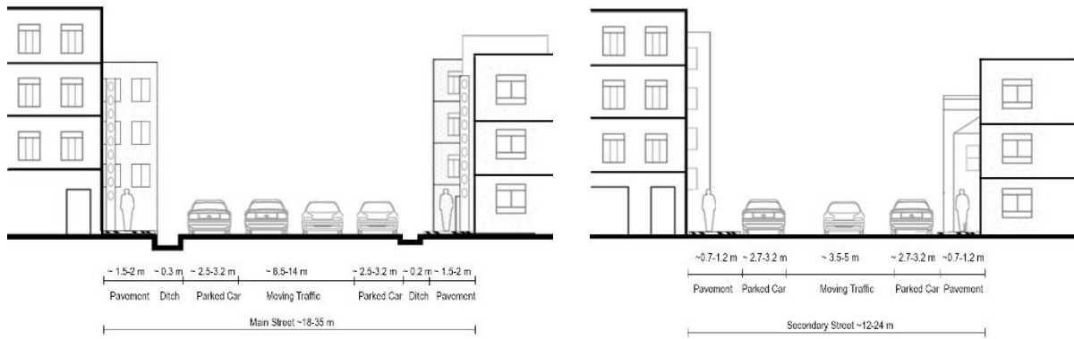
Figure 4.28. Street Section 1-1 (left) and section 2-2 (right) from main and secondary streets in Dr. Hooshyar Neighborhood
