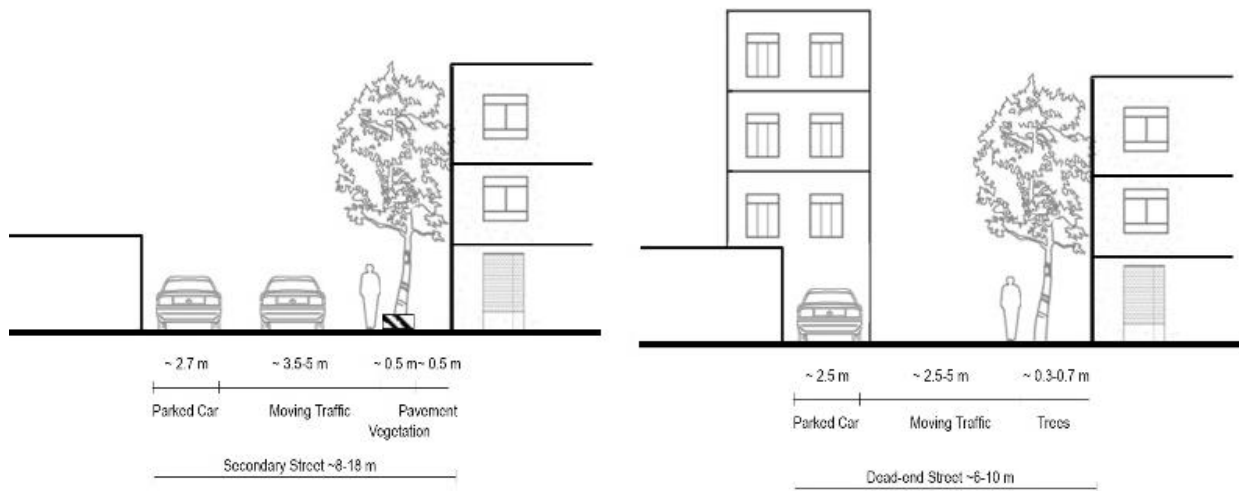
Figure 4.23. Section 3-3 (left) and section 4-4 (right) from a secondary and a dead-end street in Qeytariyeh Neighborhood
