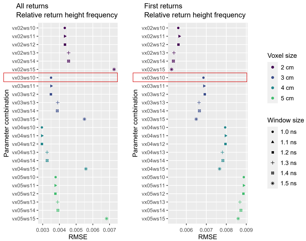
Figure 2.8: Root mean square error between simulated and observed return frequencies per 1 m height bins for different combinations of voxel size and window size applied in the HELIOS++ simulations. The red box highlights the selected parameter combination.
