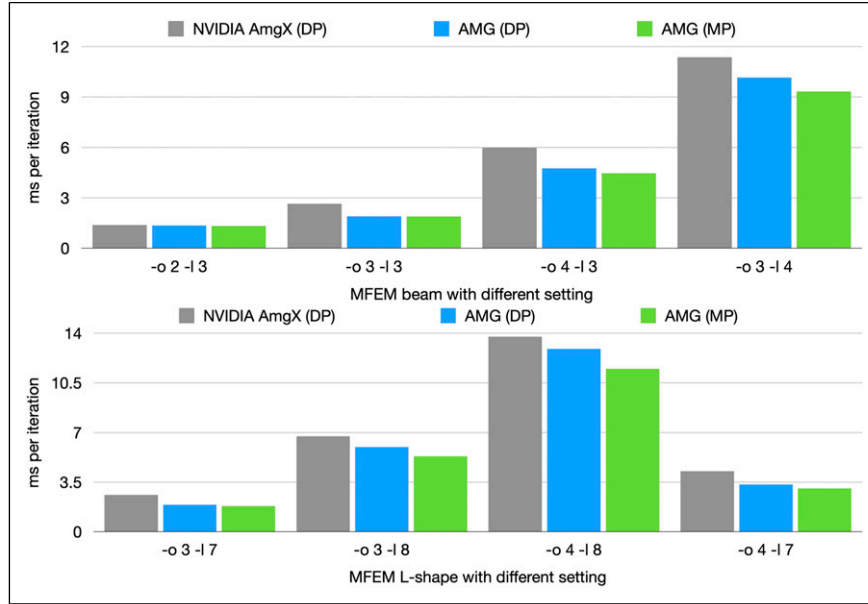
Figure 7. Runtime of one AMG-preconditioned CG iteration on the V100 GPU for MFEM's example I for the beam mesh (top) and the L-shape mesh (bottom).
