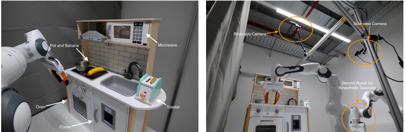
Fig. 6: Overview of the real robot kitchens setup. The left image shows the play kitchen with all its objects, while the right image shows the cameras and second robot used for data collection with our robot used for teleoperation.
